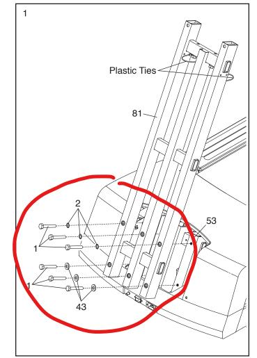
Insert the end of the Upright Wire (111) through the looped plastic tie at the top of the Upright (81). Make sure that the Upright Wire is behind the crossbars on the Upright. Then, gently pull upward on the Upright Wire as you tighten the plastic ties around the Upright Wire.
